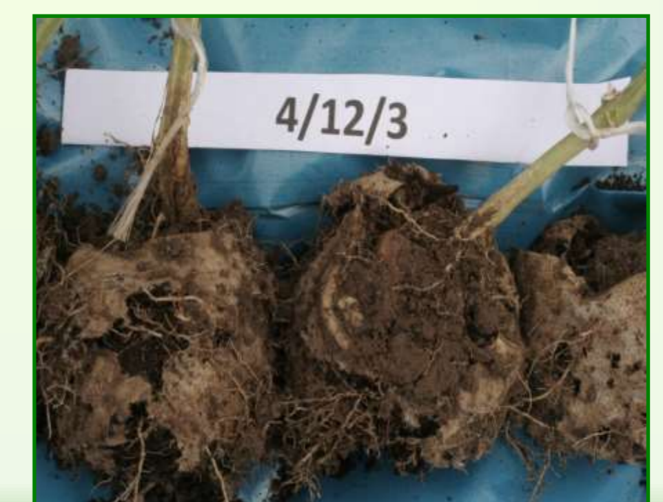
Nursery pots made from Bionolle non-woven after five weeks in the soil
