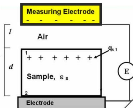
Fig. 2. Experimental setup for measuring the surface charge density: 1-, 2- surfaces of sample,  $q_{s1}$  - the surface charge density on the surface -1 of the sample
