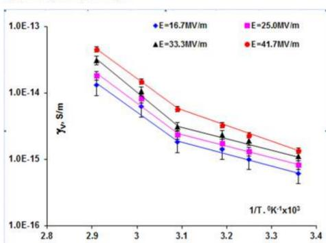
Fig. 3. Temperature characteristics of the electric conductivity of a PLA film in contact with Au electrodes. The activation energy of the charge carrier conduction reaches (0.4-0.7) eV at temperatures below the  $T_g$  and (0.9-1.1) eV at temperatures above the  $T_g$ .
