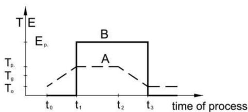
Fig. 1. Electret formation in an electric field:  $T_0$ -ambient temperature,  $T_g$ -glass transition temperature,  $T_p$ -polarization temperature,  $E(t)$ -intensity of electric field,  $E_p$ -intensity of the electric field during polarization, A-characteristics of temperature changes, B-characteristics of DC field changes.
