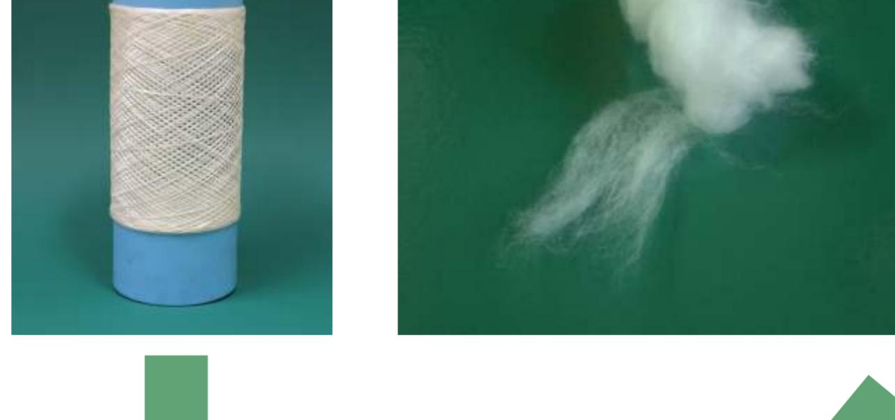
A melt-blown nonwoven was produced with surface density ranging from 50 to 150 g/m<sup>2</sup>, sorption capacity level of 4.6 g/g, with sorption rate of 3.8 µl/cm<sup>2</sup>/s .
