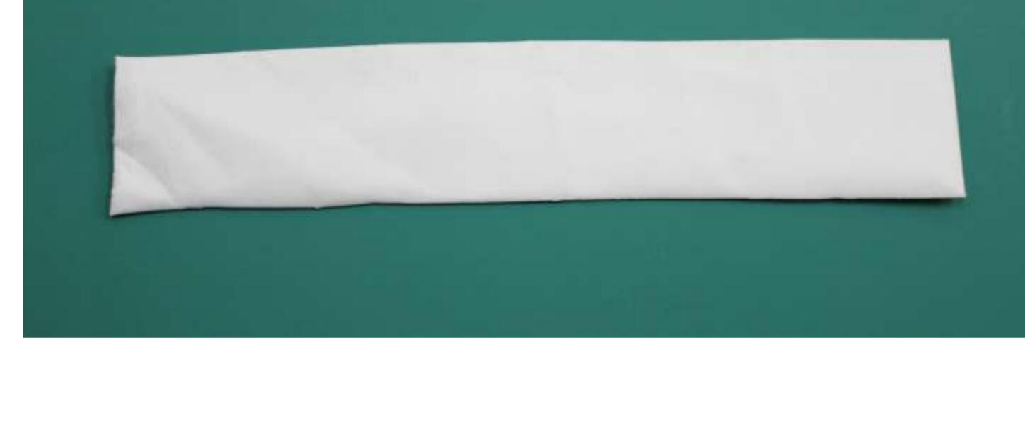
Double-layer structure of knitted fabric, with 3.72 g/m<sup>2</sup> surface density, air permeability of 5532 mm/s at 100 Pa. Elasticity 24%
