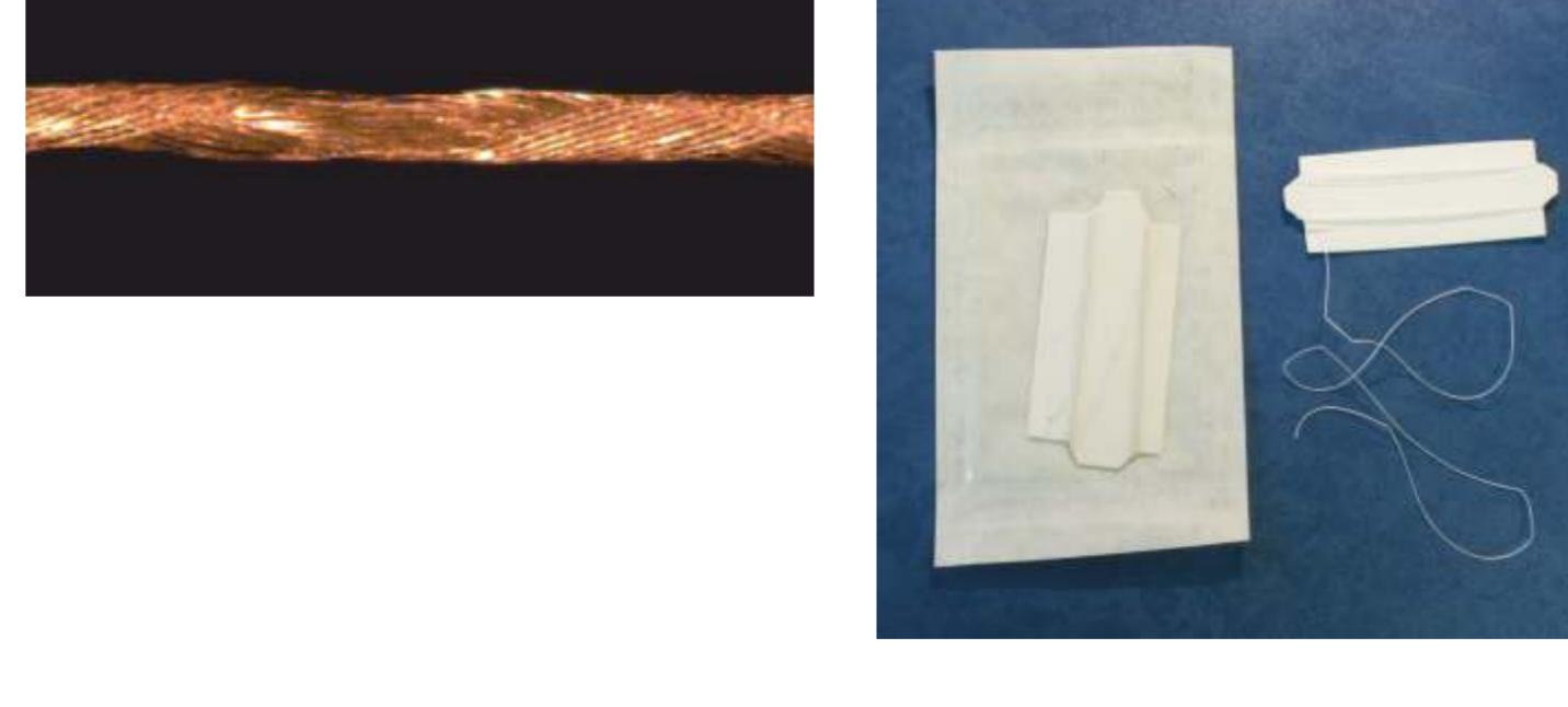
Nonwovens for bone implantation were obtained with surface density of 333 g/m<sup>2</sup>, 2.6 mm thickness, air permeability of 33 l/m<sup>2</sup>/s, sorption capacity of 8.8 g/g and sorption rate of 2.31 µl/cm<sup>2</sup>/s .
