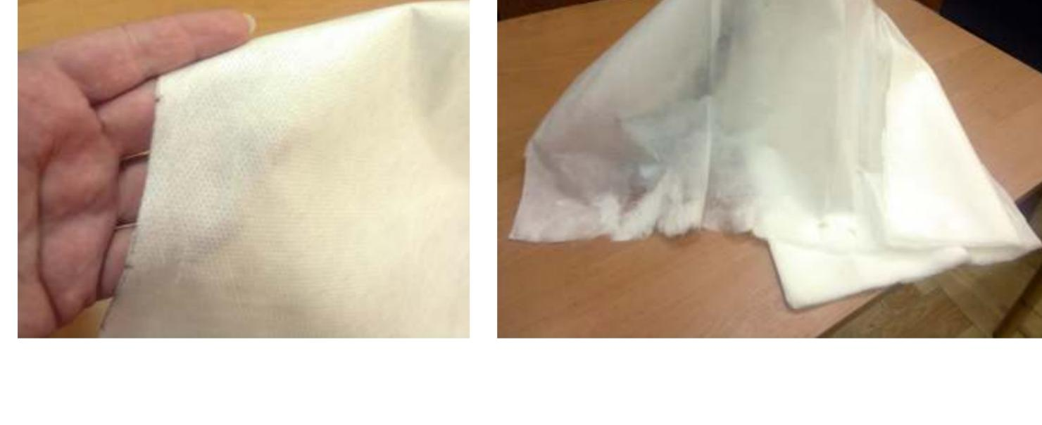
Fibres and multifilament. Multifilament was produced with linear mass at the level of 80 dtex, tenacity from 16 cN/tex and 27% elongation. Staple fibres were characterised by linear mass at the level of 7.9 dtex, tenacity from 25 cN/tex and 62% elongation.
